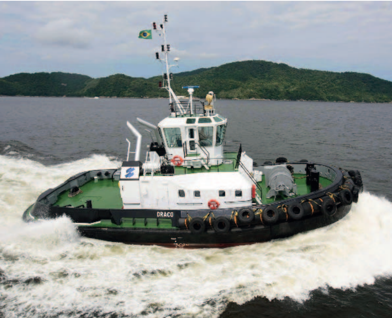
Above: The 42 ton bollard pull tug boat Draco.
